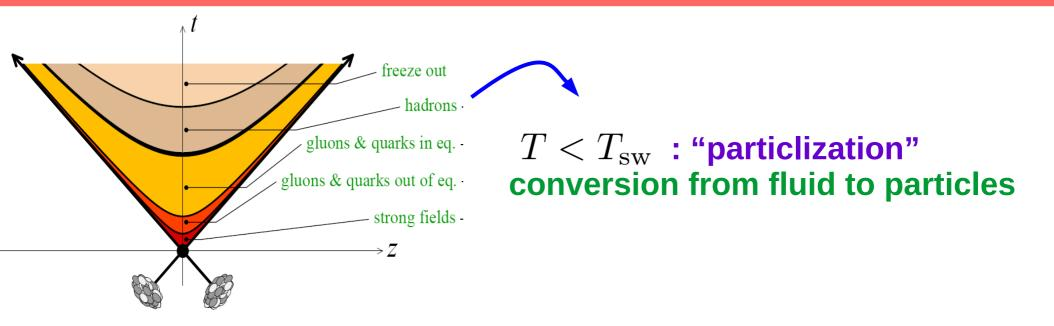
Fluid description matched to a kinetic one by sampling discrete particles along the hypersurface
